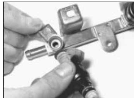
11.1 Removing a fuel injector from the rail
