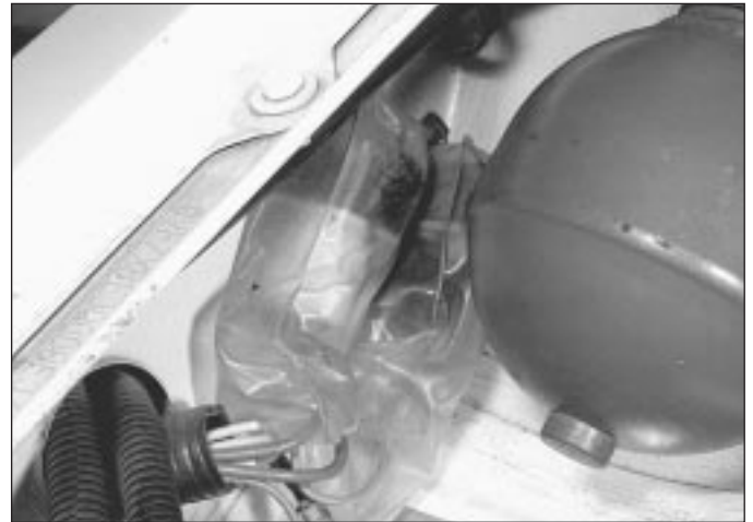
1.6b Injector and fuel pump relays protected by plastic cover - GTi 16v with Motronic ML4.1
