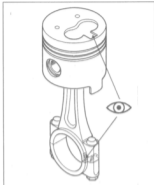
26.25A Correct piston and connecting rod assembly
