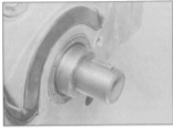
12.18 Camshaft oil seal flush with the end face of the cylinder head
