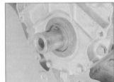
12.26 Fitting the timing belt end oil seal to the crankshaft with a plastic protector
