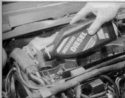
3.12c Fill the engine with the correct quantity and grade of oil
