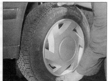
6.4 Check for wear in the hub bearings by grasping the wheel and trying to rock it
