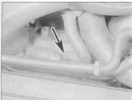
13.4c Coolant bleed screw (arrowed) in coolant bypass hose – 2.5 litre engine model
